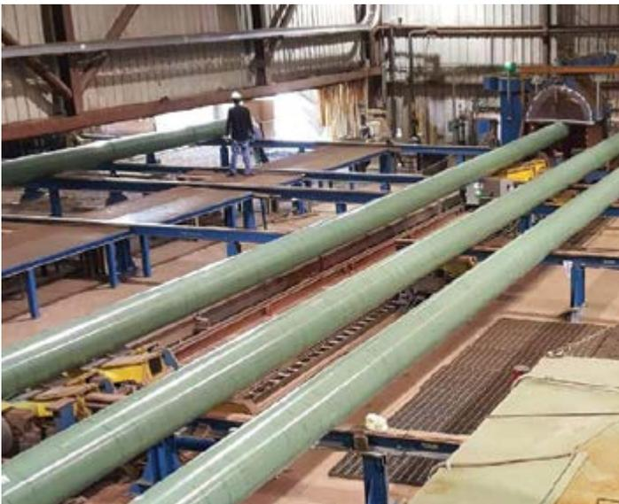
As a new offering, Flowliner coating creates a smooth surface on the ID of pipe, masking natural peaks and valleys in profiles of the steel. As the line operates at high pressures this coating mitigates turbulence in the line, facilitating laminar flow, thus reducing the friction co-efficient of the line. In turn, this lowers the compression horsepower and fuel consumption, which ultimately reduces operating cost.
